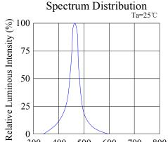
500 300 400 600 700 800 Wavelength  $\lambda p (nm)$ Luminous Intensity & **Ambient Temperature**
