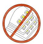
Compare to epoxy encapsulant that is hard and brittle, silicone is softer and flexible. Although its characteristic significantly reduces thermal stress, it is more susceptible to damage by external mechanical force. As a result, special handling precautions need to be observed during assembly using silicone encapsulated LED products. Failure to comply might lead to damage and premature failure of the LED.
