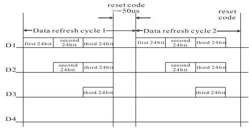
Note: The data of D1 is send by MCU, and D2, D3, D4 through pixel internal reshaping amplification to transmit.
