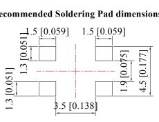
Unit: mm Tolerance: ±0.10mm
