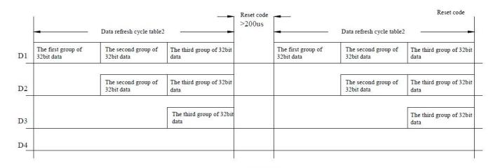
Note: The data of D1 is send by MCU, and D2, D3, D4 through pixel internal reshaping amplification to transmit.
