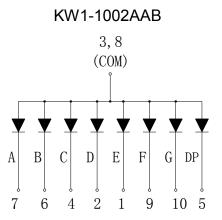
Internal Circuit Diagram (Common Cathode)
