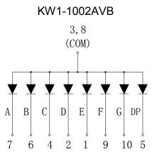
Internal Circuit Diagram (Common Cathode)
