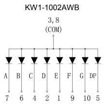
Internal Circuit Diagram (Common Cathode)
