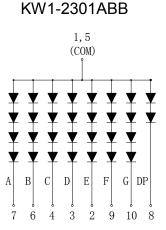
Internal Circuit Diagram (Common Cathode)
