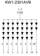
Internal Circuit Diagram (Common Cathode)
