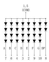
Internal Circuit Diagram (Common Cathode)
