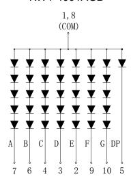
Internal Circuit Diagram (Common Cathode)
