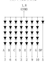
Internal Circuit Diagram (Common Cathode)
