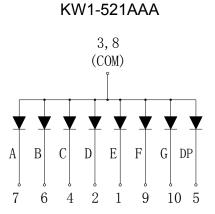
Internal Circuit Diagram (Common Cathode)
