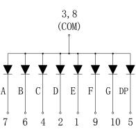
Internal Circuit Diagram (Common Cathode)
