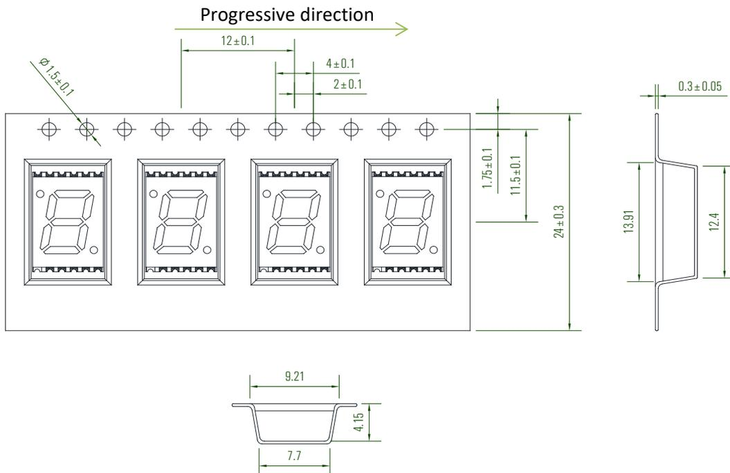
Note: Tolerances unless mentioned  $\pm 0.25\text{mm}$ .
