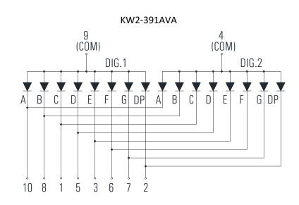
Internal Circuit Diagram (Common Anode)
