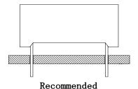
3. The component shall be placed at least 5mm from edge of PCB to avoid damage caused excessive heat during wave soldering.
