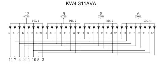
Internal Circuit Diagram (Common Anode)
