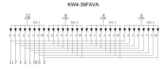
Internal Circuit Diagram (Common Anode)
