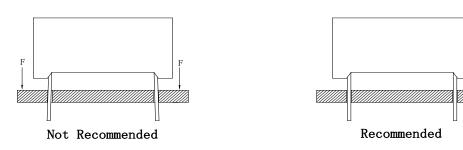
3. The component shall be placed at least 5mm from edge of PCB to avoid damage caused excessive heat during wave soldering.
