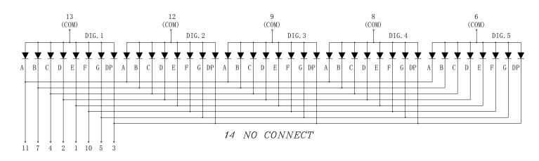
Internal Circuit Diagram (Common Cathode)
