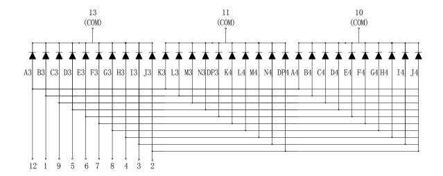
0.54 inch (13.80 mm), Orange Quadruple Digit 14-segment Alphanumeric LED Display
