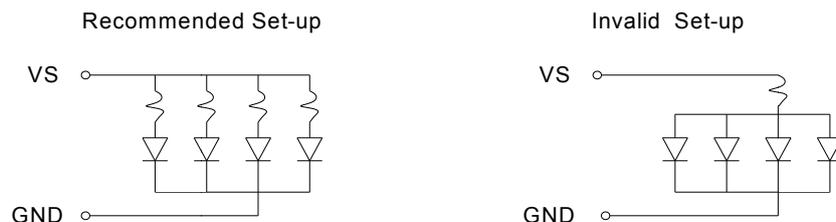
3. The driving circuit should be designed to protect the LED against reverse voltages and transient voltage spikes when the circuit is powered up or shut down.
