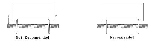
3. The component shall be placed at least 5mm from edge of PCB to avoid damage caused excessive heat during wave soldering.
