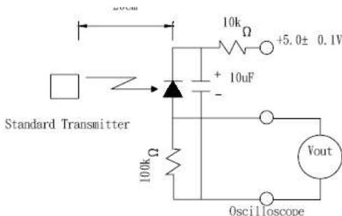
Fig.-3 Measuring System
