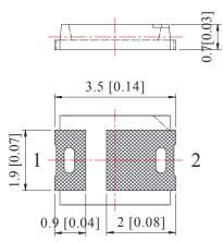
**Recommended Soldering Pad Dimensions**
