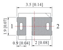
**Recommended Soldering Pad Dimensions**
