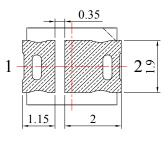
**Recommended Soldering Pad Dimensions**
