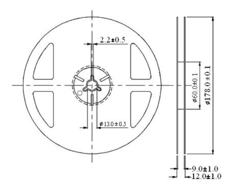
Unit: mm Tolerance:  $\pm 0.25$ mm
