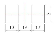
Unit: mm Tolerance: ± 0.10mm
