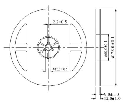
Unit: mm Tolerance:  $\pm 0.25$ mm
