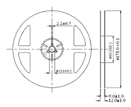
Unit: mm Tolerance:  $\pm 0.25$ mm
