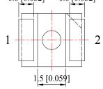
Recommended Soldering Pad Dimensions
