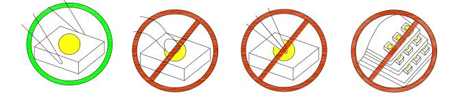
Compare to epoxy encapsulant that is hard and brittle, silicone is softer and flexible. Although its characteristic significantly reduces thermal stress, it is more susceptible to damage by external mechanical force. As a result, special handling precautions need to be observed during assembly using silicone encapsulated LED products. Failure to comply might lead to damage and premature failure of the LED.
