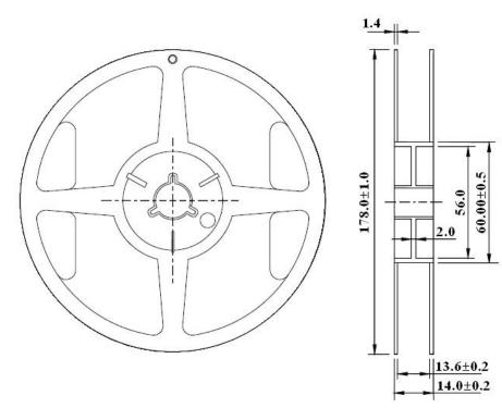
Unit: mm Tolerance: ±0.25mm
