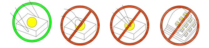
1.4 Compare to epoxy encapsulant that is hard and brittle, silicone is softer and flexible. Although its characteristic significantly reduces thermal stress, it is more susceptible to damage by external mechanical force. As a result, special handling precautions need to be observed during assembly using silicone encapsulated LED products. Failure to comply might lead to damage and premature failure of the LED.
