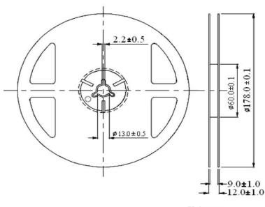
Unit: mm Tolerance:  $\pm 0.25$ mm
