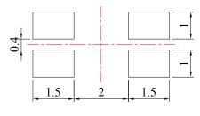
Unit: mm Tolerance:  $\pm 0.10$ mm
