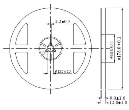
Unit: mm Tolerance: ±0.25mm
