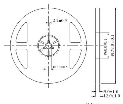
Unit: mm Tolerance: ±0.25mm
