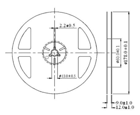
Unit: mm Tolerance:  $\pm 0.25$ mm
