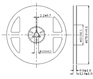
Unit: mm Tolerance:  $\pm 0.25$ mm
