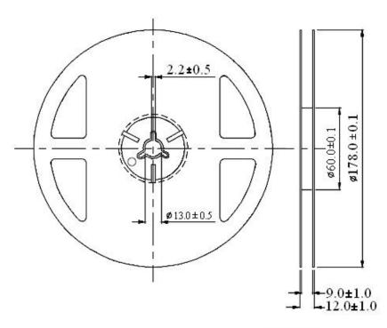
Unit: mm Tolerance:  $\pm 0.25$ mm
