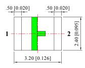
**Recommended Soldering Pad Dimensions**
