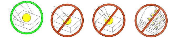
Compare to epoxy encapsulant that is hard and brittle, silicone is softer and flexible. Although its characteristic significantly reduces thermal stress, it is more susceptible to damage by external mechanical force. As a result, special handling precautions need to be observed during assembly using silicone encapsulated LED products. Failure to comply might lead to damage and premature failure of the LED.
